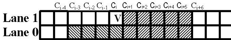
Fig. 7. Example of 2 lanes highway. The vehicle being considered is located at cell c_i on Lane 1. Its neighbourhood consists of two parts: the forward tilted lines show “Forward Neighbourhood”(consisting of cells c_{i+1} , c_{i+2} , c_{i+3} , c_{i+4} , and c_{i+5} on lanes 0 and 1), while backward tilted lines show “Backward Neighbourhood” (consisting of cells c_i , c_{i-1} , c_{i-2} , and c_{i-3} on lane 0).
